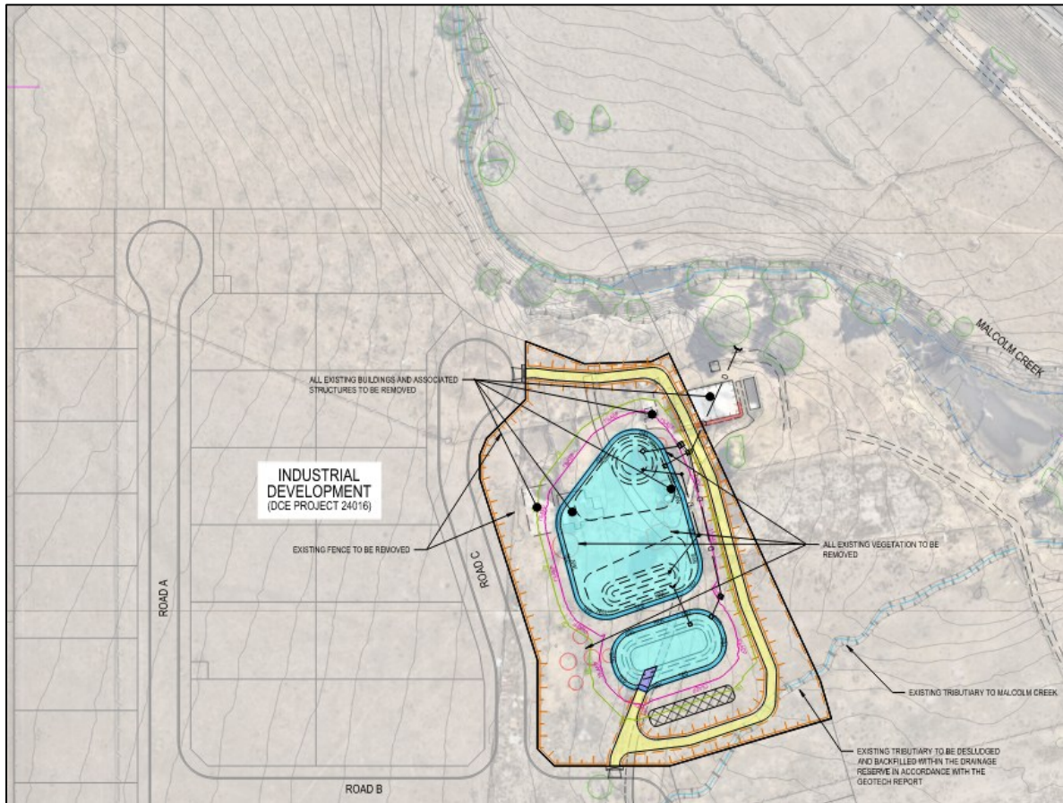
Plate 13. Proposed location of the stormwater sediment basin in the northeast corner of the study area. Image supplied by the proponent.
