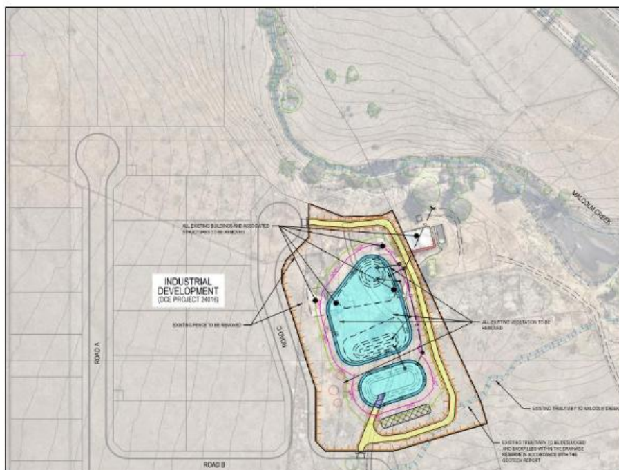
Plate 13. Proposed location of the stormwater sediment basin in the northeast corner of the study area. Image supplied by the proponent.
